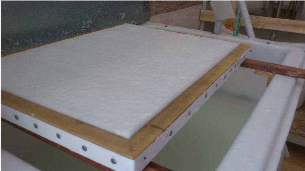
**A watery sheet of handmade paper just lifted up from vat (YAK Handmade Paper)**
